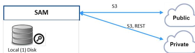
For organizations requiring higher levels of availability SAM can be deployed in an Active-Active or Active-Passive pair. SAM can also be deployed in a 3 node or larger cluster with all nodes being Active.
